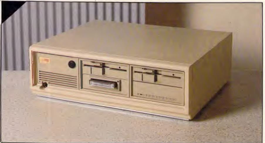
The 386 provides four slots in one unit, including a 40Mbyte tape streamer
